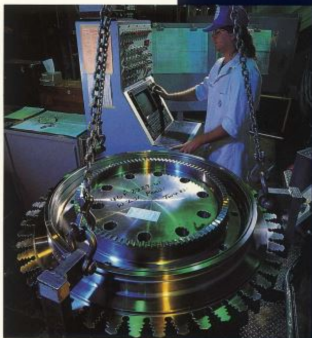
top: Metal-to-metal surfaces are machined to a precision finish by the computer numerically controlled planomill.
