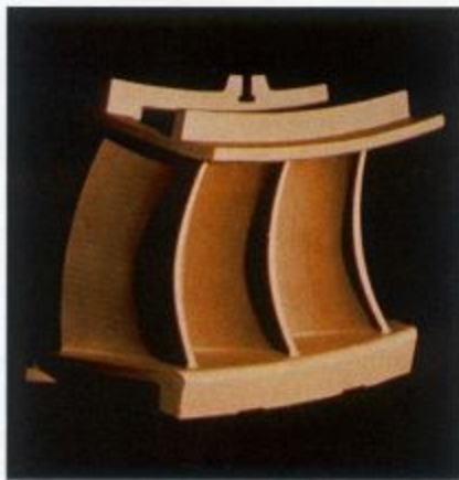
Vanes segment for the third stage is precision-cast X45 material, cooled by compressor bleed air from the 10th stage. Third stage is made up of 16 of these three-vane segments.
