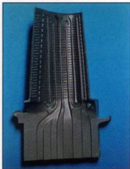
Air-cooled first stage turbine blades use combination of impingement, film and pin-fin cooling techniques to keep average metal temperatures below 1470°F at base load turbine inlet temperature of 2300°F.
