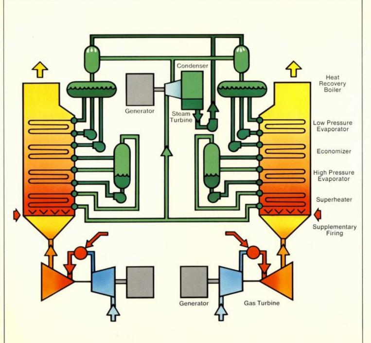
the evaporative and superheater sections to generate steam. This steam is piped to a steam header which supplies the steam for the steam turbine.
