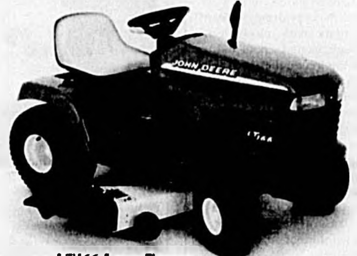
LT166 Lawn Tractor • 16-hp engine • 42- or 46-inch mowing deck • Automatic transmission
