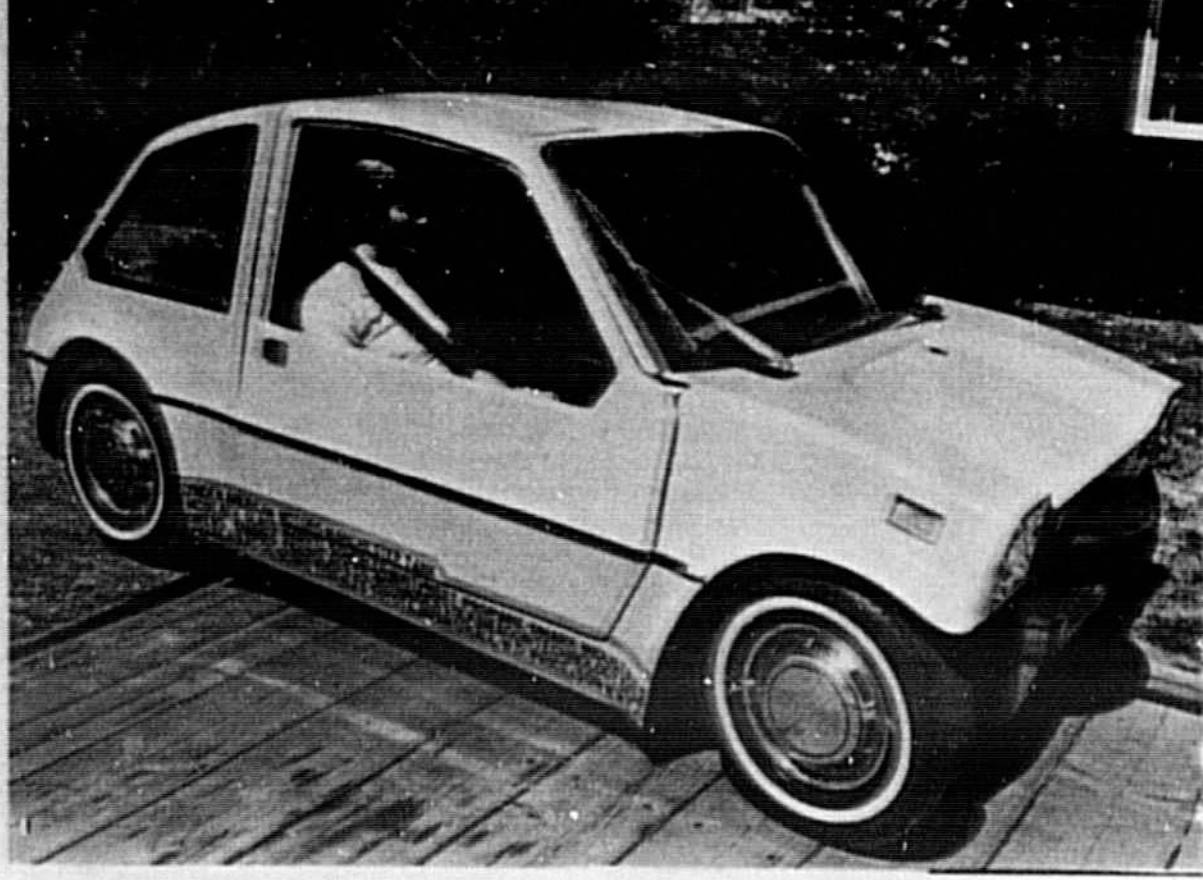
'SMOGLASS' CAR — This 16-foot-long, two-seat auto was built by students at Western Washington State College in an effort to help solve the pollution problem. The car has a rear-mounted, four-cylinder engine, which burns propane. It will comply with federal pollution standards for 1976.
