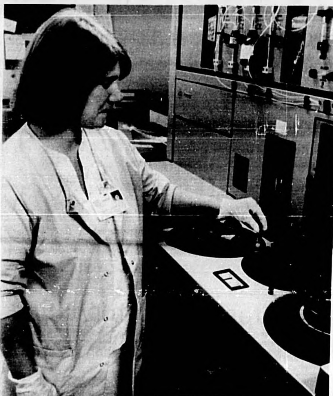
Sandy Begala, a lab technician at Central Florida Regional Hospital, uses a Paramax machine. The device is a chemistry analyzer used in testing blood for viruses and other contaminants.
