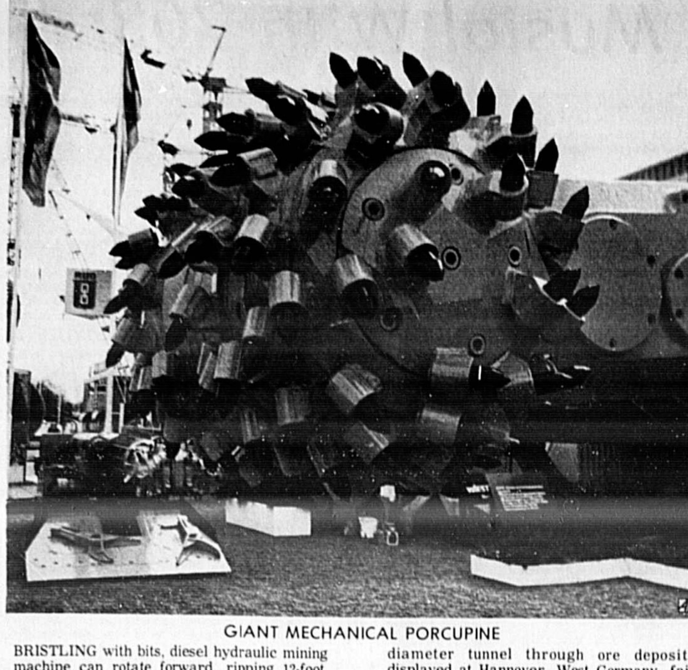
BRISTLING WITH bits, diesel hydraulic mining machine can rotate forward, ripping 12-foot diameter tunnel through ore deposits, displayed at Hannover, West Germany, fair.
