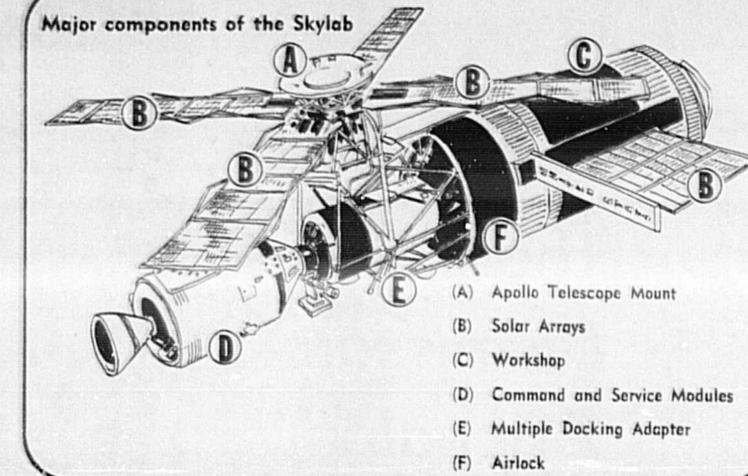
Skylab is a 67-foot-long orbiting space station in which three-man astronaut crews will live and work for periods of 28 to 56 days. It has three times as much usuble space as the Apollo command module used in
