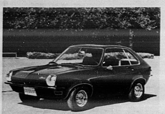
EXPERIMENTAL ONLY — This is the General Motors special purpose vehicle, the XP-883, designed to use gasoline, electric or hybrid gasoline-electric power systems.
