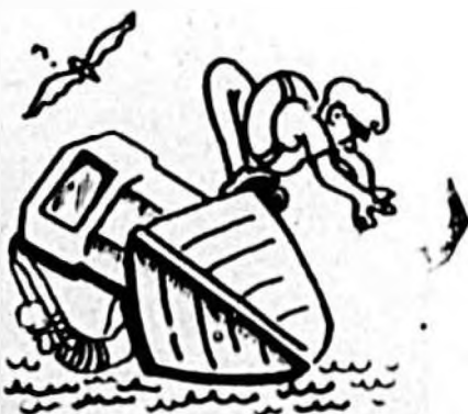
Smashed in bow of the sturdily built steel cabin cruiser (above) was result of head-on collision with a causeway because the operator became "rattled" when engine throttle button was stuck, while cruising in restricted waters.
