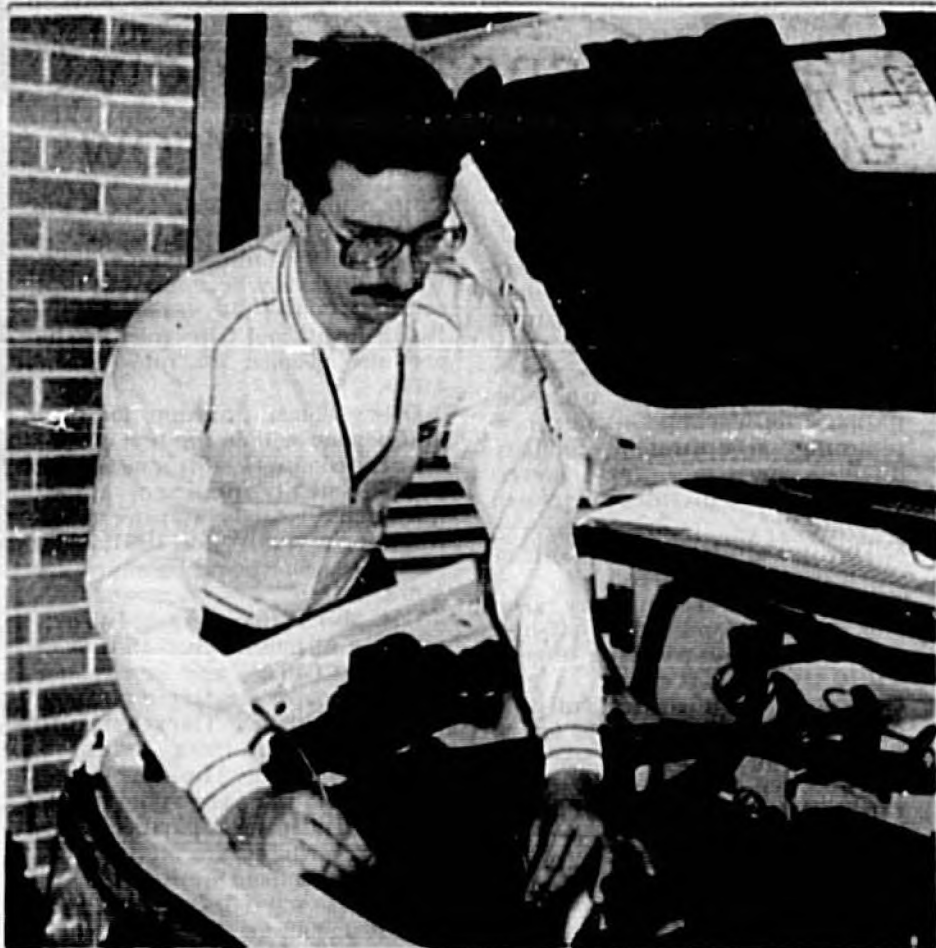
Owners should note condition of belts, hoses and wiring.
