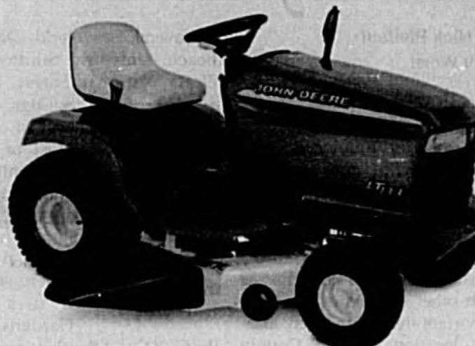
LT133 Lawn Tractor • 13-hp engine • 38-inch mowing deck • 5-speed transmission
