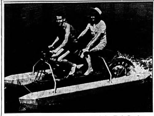
THE BICYCLE built-for-two has gone nautical. An Illinois firm has a patent pending on this two-seater, propelled by twin metal paddle-wheels operated otherwise like a regulation bicycle.
