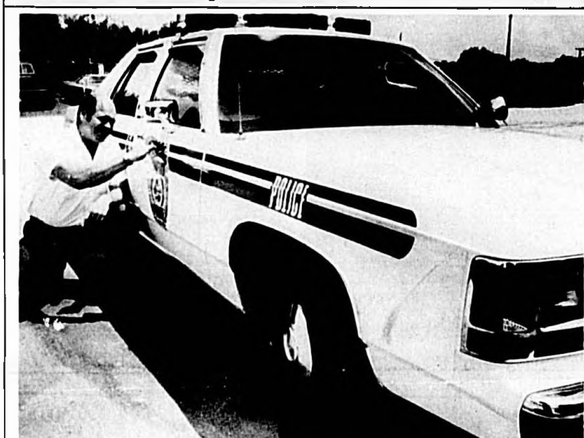
Wayne Bally, City of Sanford lead mechanic applies Police decals to a police car sporting a new design. Use of decals over painted emblems saves the city over $700 per vehicle.
