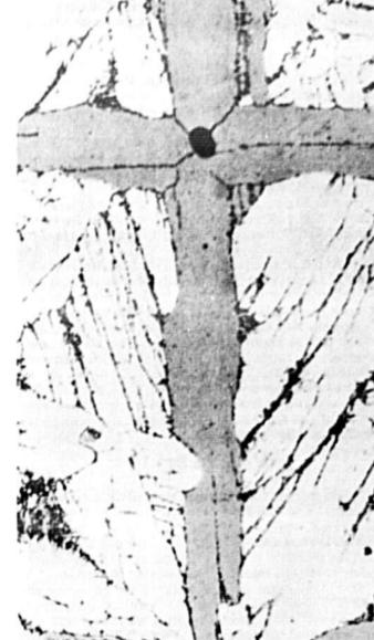
season, this cross comes not from an artist's brush but from a microscope. It is a tiny speck of zirconium alloy magnified 300 times at laboratories in Schenectady, N.Y., of the General Electric Research and Develop-
