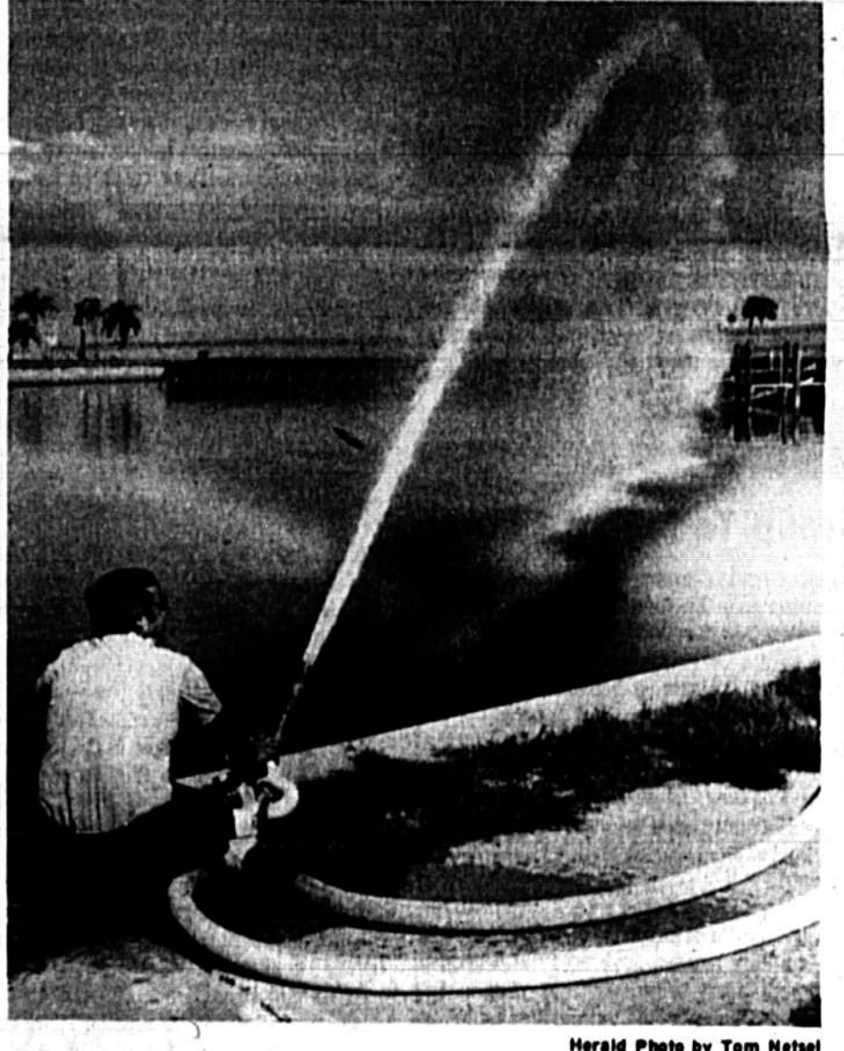
SPRAY DAY Firefighter Mike Hoening of the Sanford Fire Department drafts water from Lake Monroe at the Sanford Marina as he does periodic check to make sure the pumper truck is working at its capacity of 750 gallons a minute. With the latter at such a low level the firemen barely had enough water for the test.
