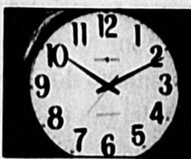
This radio-controlled clock receives a signal four times per day that keeps it in sync with the atomic clock, the world's most accurate clock.
