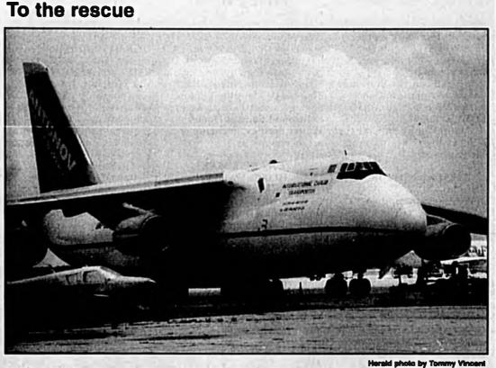
A giant cargo plane owned by Antonov International Cargo Transport dwarfs alreraft at the Orlando Sanford International Airport. The plane transported a fully assembled jet engine from Europe for a JMC Airliner that experienced an engine malfunction.
