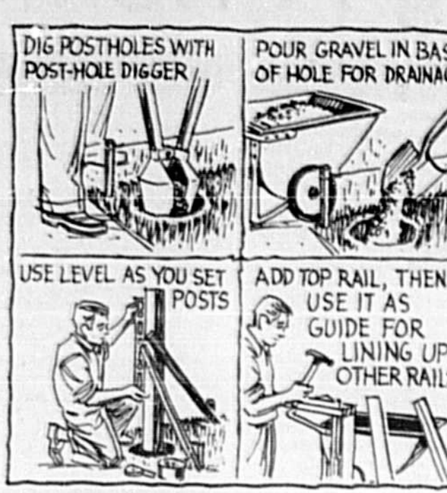
DIG POSTHOLES WITH POST-HOLE DIGGER. POUR GRAVEL IN BASE OF HOLE FOR DRAINAGE.
