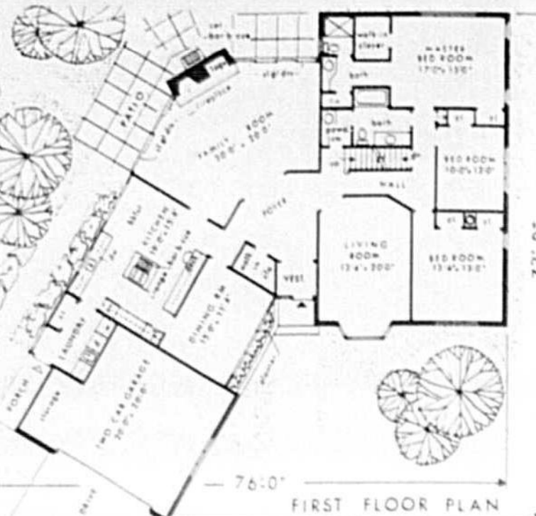
THE DRAMA of unfolding space is created at the intersection of two angled wings where a triangular foyer leads to an expanding fan-shaped family room...
