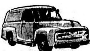
NEW longer springs and new tubular tires in Ford "1/2-ton" Series give softer ride for driver and load. Shown new Ford F-100 8-Ton Panel, GVW 5,000 lbs.
