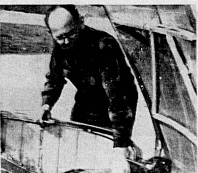
ELECTRIC AUTO . . . J. E. McAlexander Jr. of Sanford has converted a small model auto into an electric (battery operated) auto as a hobby. "Mac" is shown examining his power sources — four batteries under the hood and a converted battery charging generator in the back end. Although it is quiet, the vehicle is also quite expensive — getting just four miles before batteries must be recharged. (Herald Photos)
