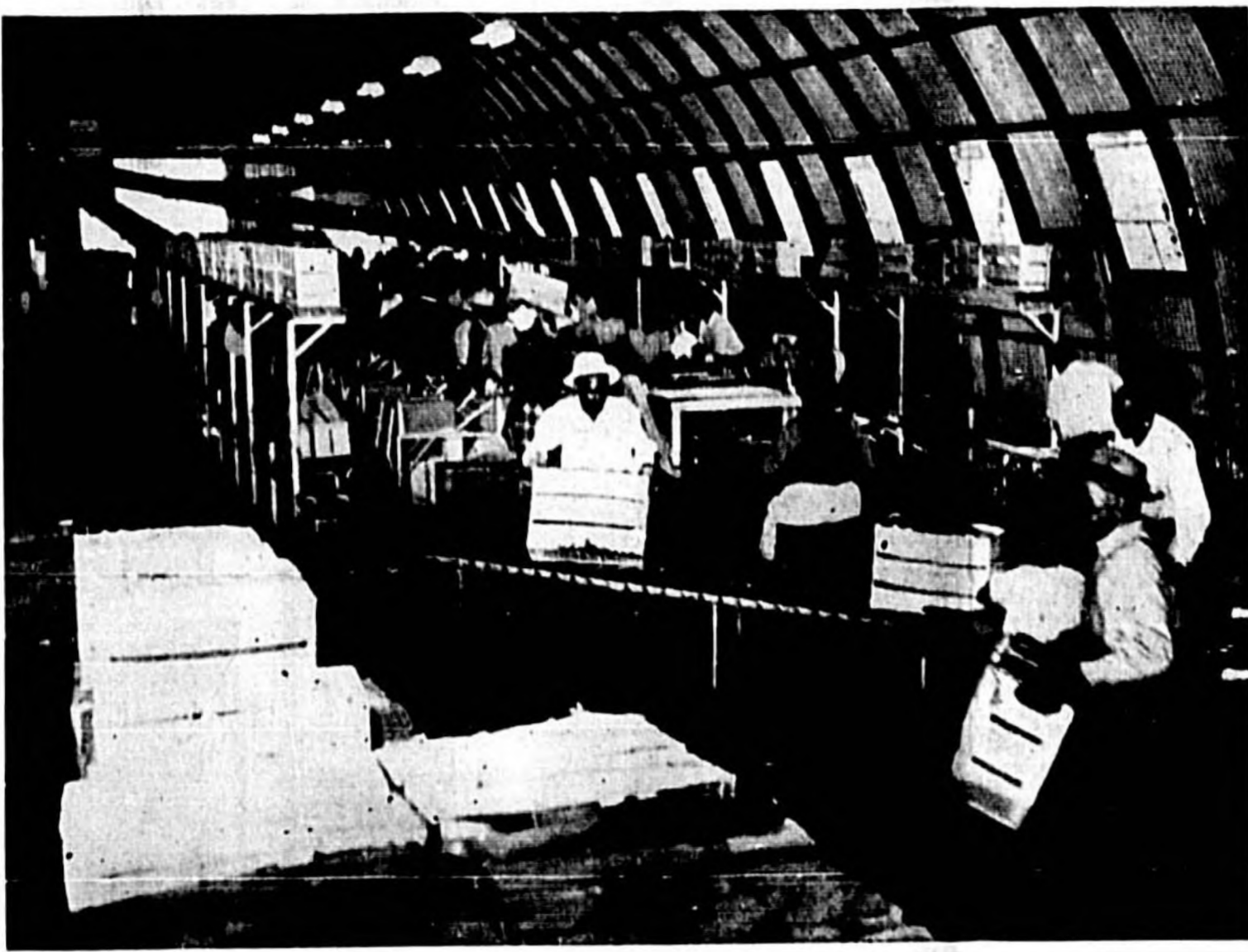
Workers are shown at the new Grapeville Avenue plant of American Fruit Growers Inc. on the west side which was recently completed and put into operation. Workers in the foreground are stacking the washed and packed celery. From there it will go on belt lines to the pre-cooler and to refrigerator cars. The crates for packing are shown on overhead racks to where they roll from an overhead station. On the other side of the building is a like scene of packing activity.
