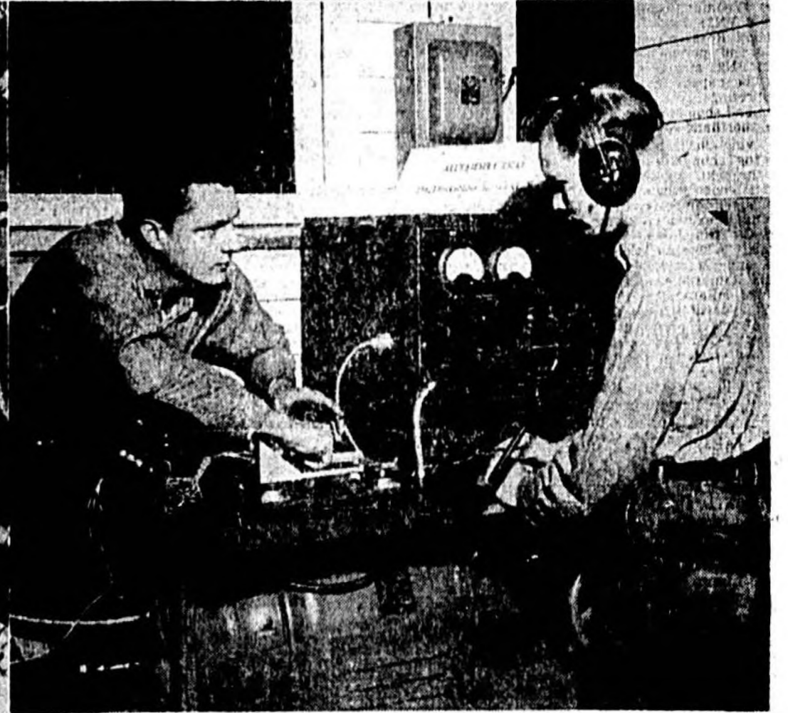
SOME OF THE most important and detailed work in the entire Fleet Aircraft Squadron at the Naval Auxiliary Air Station takes place in the electronics shop. Above is shown James H. Himes, AEN at the left with James C. Carter, AEAN, on the right. They are shown setting up a voltage regulator for a torpedo Bomber.
