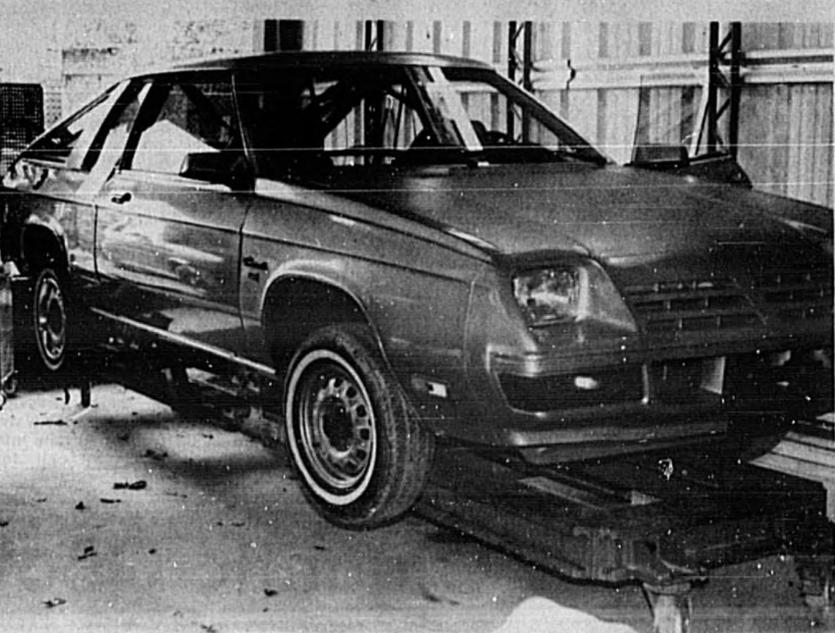
The Car-o-liner at Seminole Paint and Body aligns car's unitized chassis within three millimeters of factory specifications.
