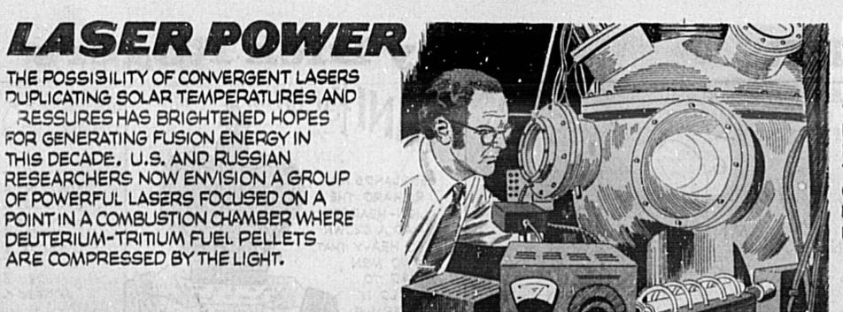
EACH PELLET OF THE DEUTERIUM-TRITIUM MIXTURE -ABOUT THE SIZE OF A PINHEAD-WOULD BE DROPPED INTO THE BLAZING FOCUS POINT WHERE THE IMMENSE FORCE OF THE PULSED LASER LIGHT WOULD COMPRESS IT FROM ALL SIDES.
